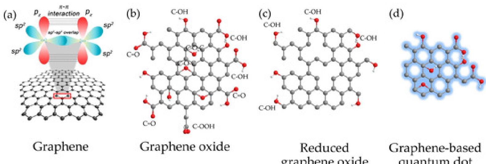
Structures of graphene-based materials show (a) the pristine graphene (pure-arranged carbon atoms) with  $sp^2$ -hybridized carbon atoms, and the chemically modified graphene, including (b) graphene oxide (GO); (c) reduced graphene oxide (RGO) and (d) graphene quantum dot (GQD).
