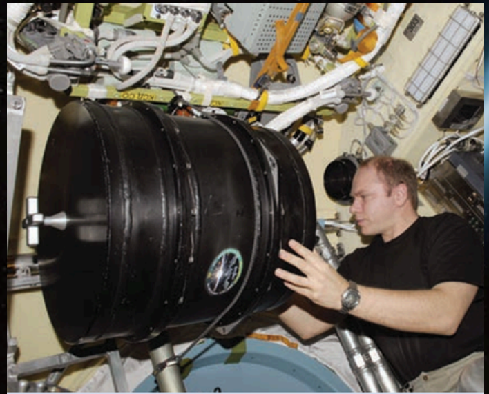
Russian cosmonaut Oleg Kotov, Expedition 30 flight engineer, inspects the Plasma Kristall Experiment laboratory, enclosed in black housing, in its new home in the Poisk Mini-Research Module 2 of the International Space Station.
